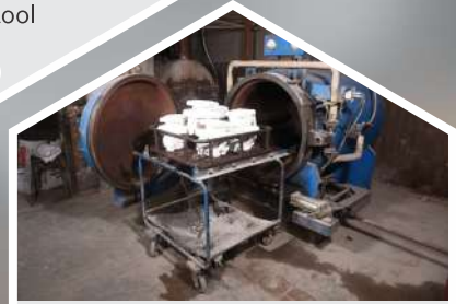
DE-WAXING Removing wax from Shell by auto-clave
