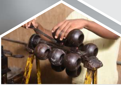
METHODING Attachment of patterns with feeders
