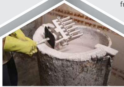
CERAMIC COATING Application of coatings with binder & stucco
