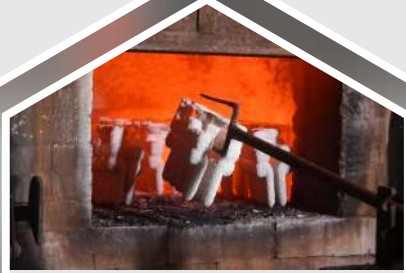
SHELL PRE-HEATING Pre-Heating of shells
