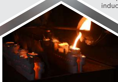
POURING Filling the shells with molten metal
