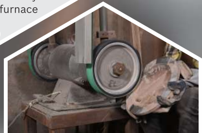
FETTLING Detachment from feeders and surface finishing
