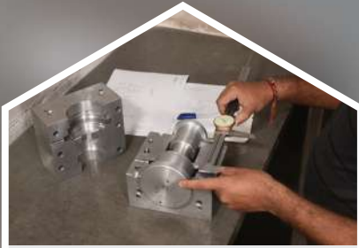
TOOL DEVELOPMENT Tool established for making wax patterns
