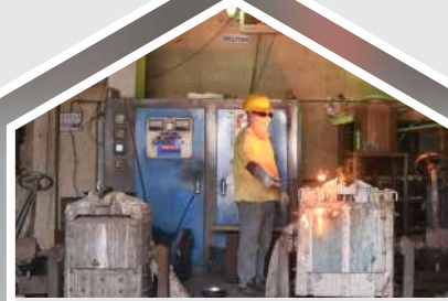
MELTING Preparation of liquid metal by induction furnace
