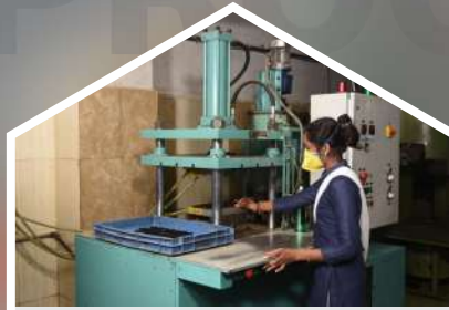
WAX PATTERN MANUFACTURING Output of wax injection from tool
